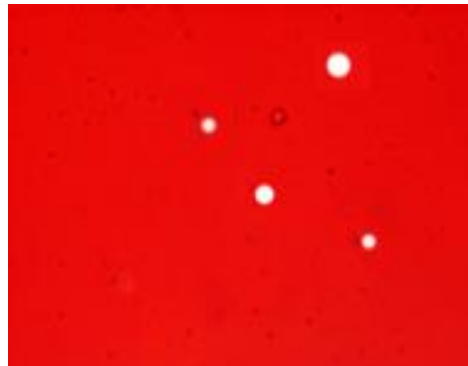
Figure 10: Photograph of Alpha tracks in LR -115 Detector for Sample (S2)
