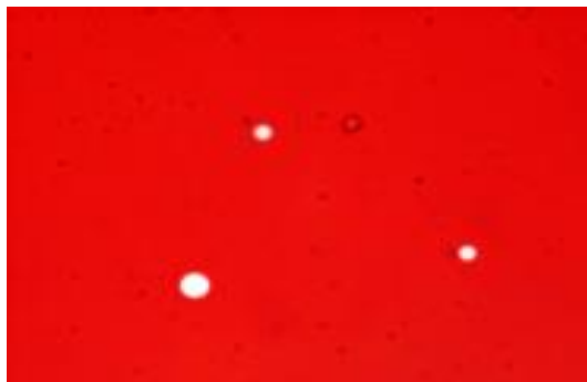
Figure 11: Photograph of Alpha tracks in LR-115 Detector for Sample (S3)
